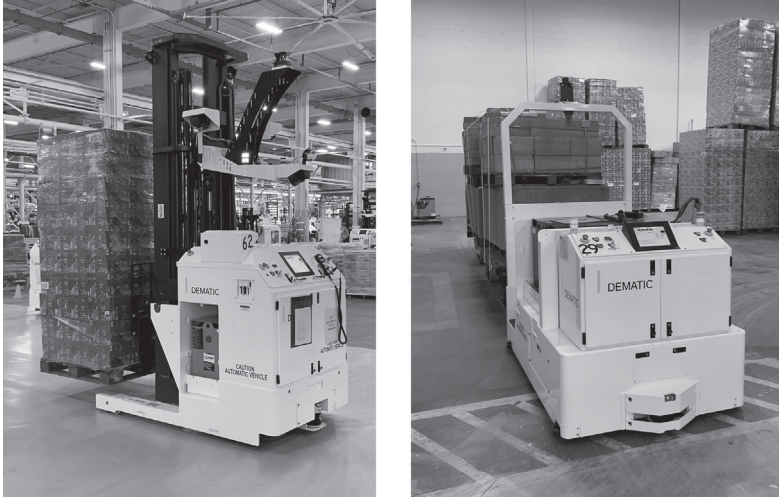
Figure 11.1 A Forklift AGV is shown on the left, and a tugger AGV is shown on the right, both offered by Dematic. © 2023 by Dematic Corp
