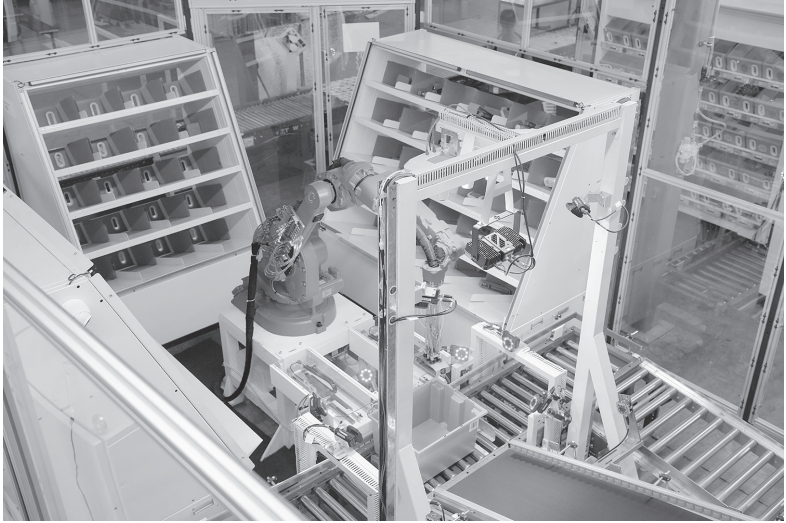
Figure 6.6 A GTR picking cell developed by Covariant, shown picking items from arriving donor totes and depositing them into a Put Wall. © 2023 by Covariant
