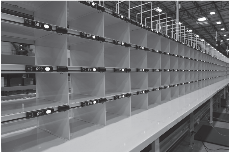
Figure 7.2 A put wall from Matthews automation, with an illuminated light identifying the slot where the current item is to be placed. © 2023 by Matthews Automation Solutions
