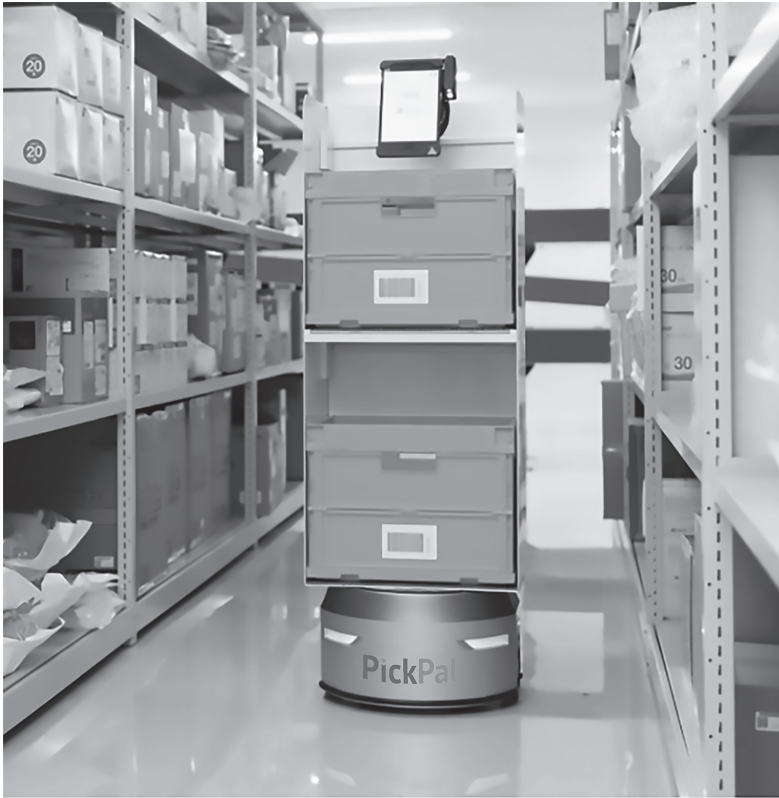
Figure 6.3 AMR-assisted Person-to-Goods picking using PickPal from Tompkins Robotics. © 2023 by Tompkins Robotics
