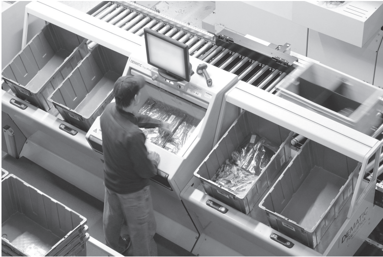
Figure 6.5 Four-order, high-speed pick station from Dematic. © 2023 by Dematic Corp
