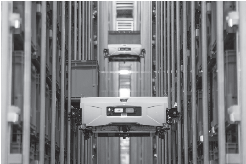
Figure 5.5 Exotec's Skypod system, showing multiple Skypods within the racking structure. After retrieving a designated tote, the bots exit the rack and deliver the totes to dedicated picking stations. © 2023 by Exotec
