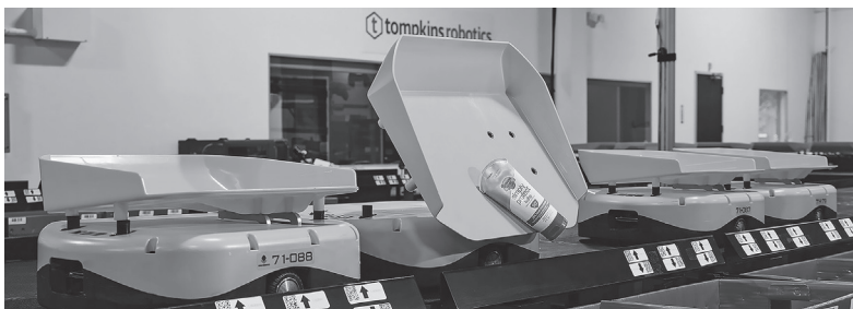
Figure 8.3 Tompkins Robotics’ t-Sort sortation solution using a swarm of Tilt-tray enabled AMRs. © 2023 by Tompkins Robotics
