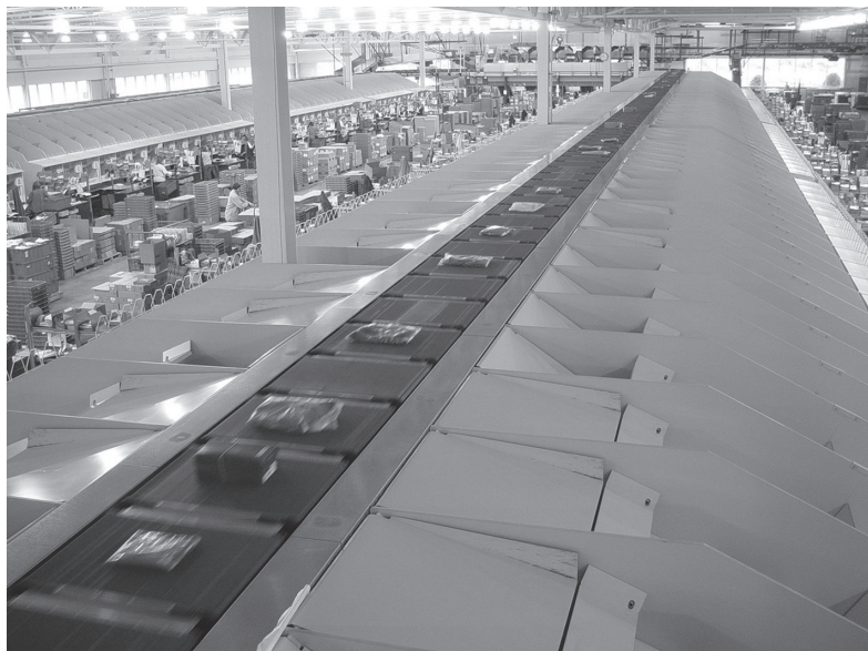
Figure 7.1 A dual-sided crossbelt sorter from Dematic. © 2023 by Dematic Corp
