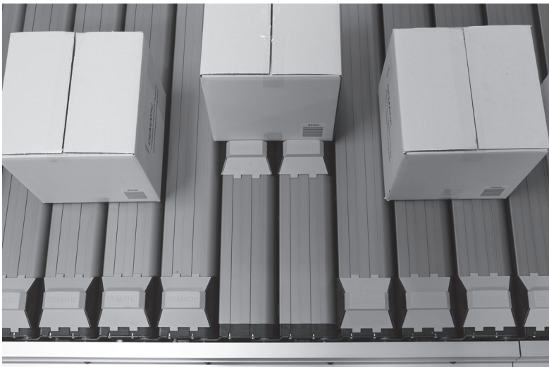
Figure 8.2 Dematic's FlexSort SL2 sorter, showing the driven chain, the parallel slats, and the mounted shoes. © 2023 by Dematic Corp
