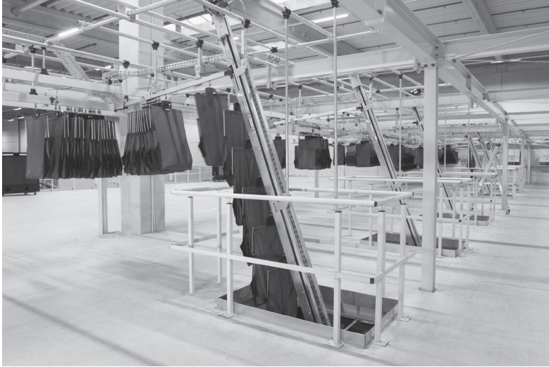
Figure 5.8 Pouch sorter from Dematic. © 2023 by Dematic Corp
