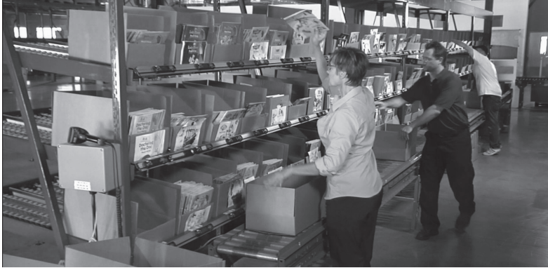
Figure 6.2 Simple manual conveyor-based pick-to-light, PTG solution from Matthews Automation. © 2023 by Matthews Automation Solutions
