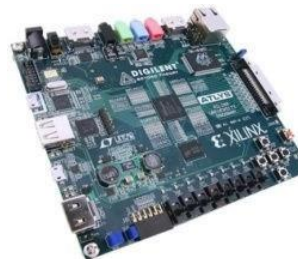
Gambar 4.18 Spartan-6 XC6SLX45 CSG324C [10]
