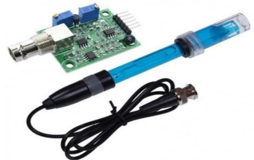
GAMBAR 5 SENSOR PH 4502C
