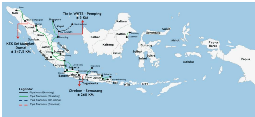
Figure 1.2 Transmission Gas Pipeline [19]
