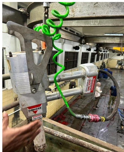
Gambar I.5 Jenis Pneumatic Stunner di RPH Ciroyom Depot
