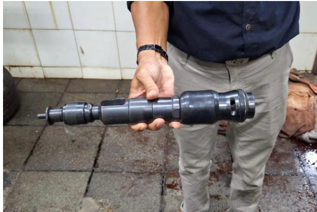
Gambar I.4 Jenis captive bolt stunner di RPH Ciroyom Depot
