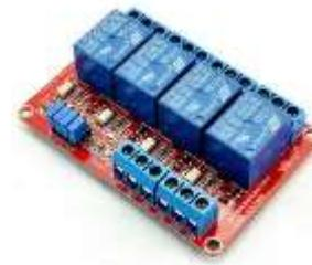
Gambar 4 Relay 4 Channel
