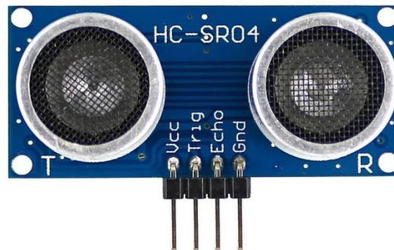
Gambar 2.2 Sensor Ultrasonik
