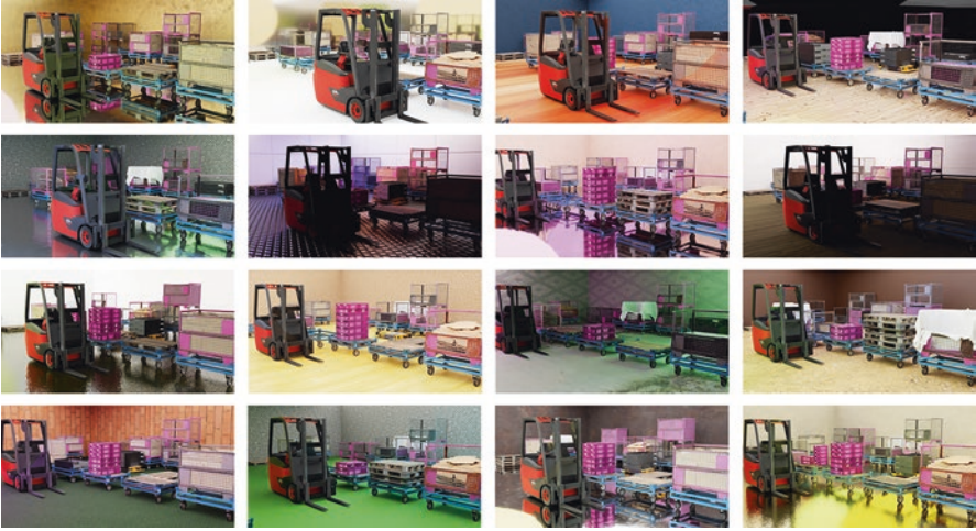
Fig. 8.2 Mixture of domain randomization components from a static camera viewport using SORDI assets [7]
