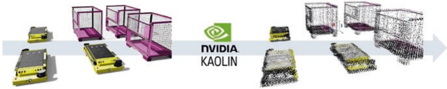
Fig. 3.6 Generating SORDI 3D point cloud assets using NVIDIA Kaolin
