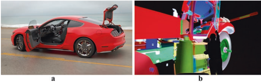
Fig. 4.5 Sample digital twin auto models. (a). High-resolution rendering of a Ford Mustang auto [25]. (b). A user checking the door handle location of a large tractor at Case New Holland [25]
