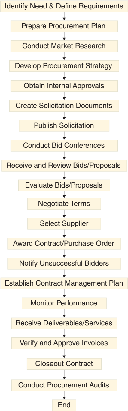
Figure 2.25 Flowchart of the procurement process
