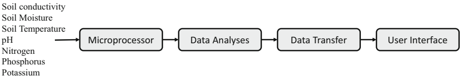
Fig. 5. Design Flow of the Sana Solo System.
