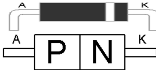
Gambar 2. 2 Penjelasan Kaki Dioda [14]
