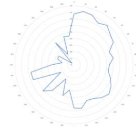
Figure 4.6 6 GHz Azimuth Radiation Pattern.
