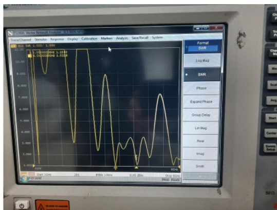
Figure 4.2 The results of the VSWR using VNA.
