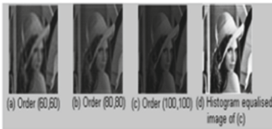
Fig. 9. Reconstruction of image using fast legendre moments of various order followed by histogram equalization
