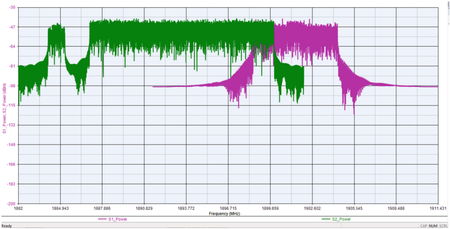
Fig. 3. Test of the spectrum during the coexistence of 4G LTE and 5G NR. ( f_1 = 1.901 GHz, f_2 = 1.892 GHz)
