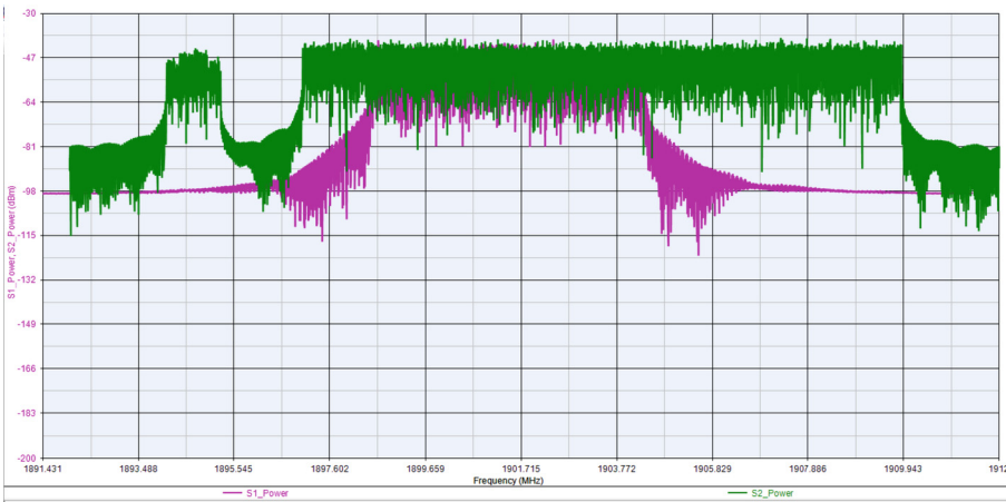
Fig. 5. Test of the spectrum during the coexistence of 4G LTE and 5G NR. ( f_1 = 1.901 GHz, f_2 = 1.902 GHz)
