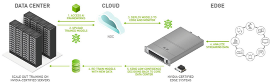
Fig. 1. Lifecycle of an edge AI application
