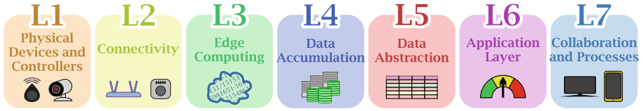
Fig. 1. Seven IoT architecture levels according to WFRM [4].
