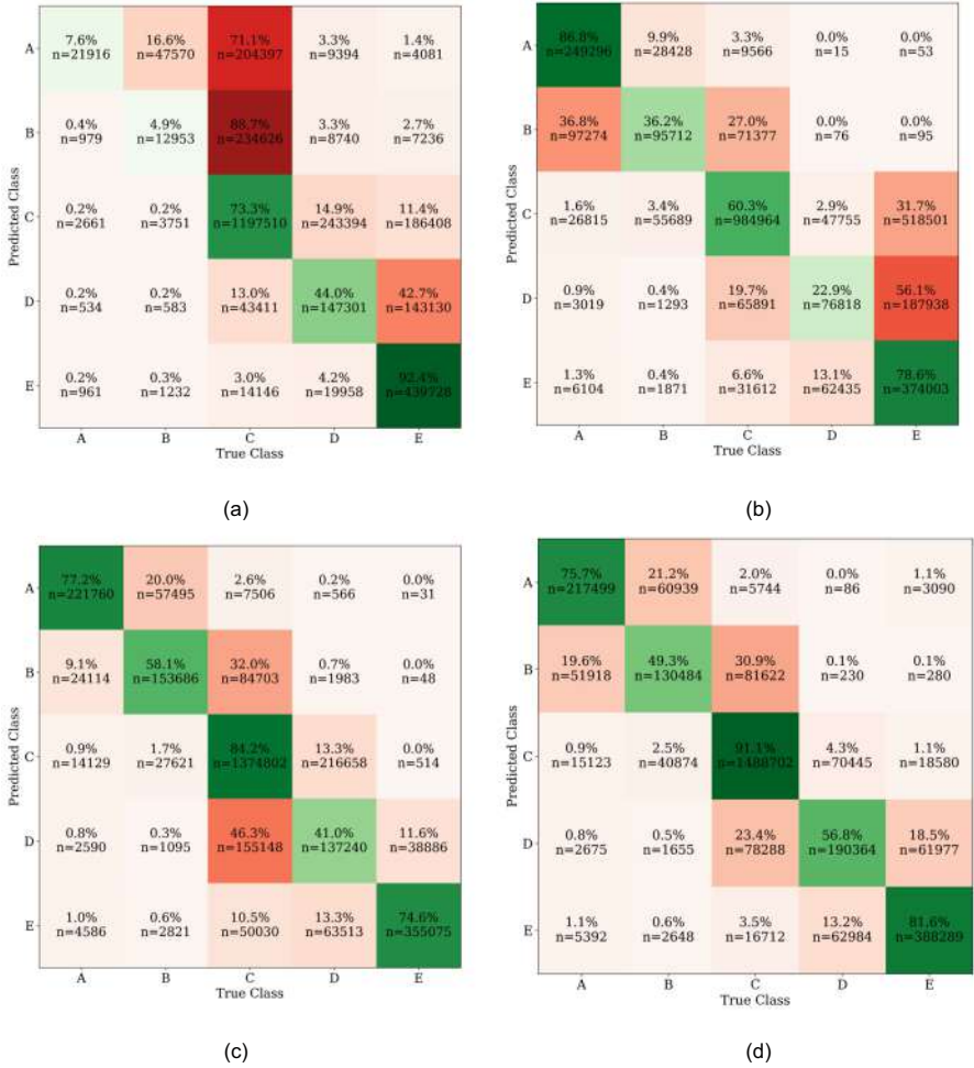
Fig. 7. Confusion Matrices of (a) CNN-MLP: Node features from the CNN encoder are directly given to the MLP for classification, (b) GNN-MLP: Node feature vectors are obtained from a linear layer instead of the CNN encoder are passed on to the Nodeformer and MLP for classification, (c) our complete model, and (d) our model with the CNN encoder initialized with the VertNormPred pre-trained weights. Labels A: ( < -0.16 mm), B: ( -0.16 mm to -0.1 mm), C: ( -0.1 mm to 0.1 mm), D: ( 0.1 mm to 0.16 mm), E: ( >0.16 mm).
