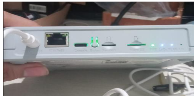
GAMBAR 7 Interface Gateway Sensecap LoRAWAN
