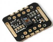
GAMBAR 2 Pulse Sensor MAX30102
