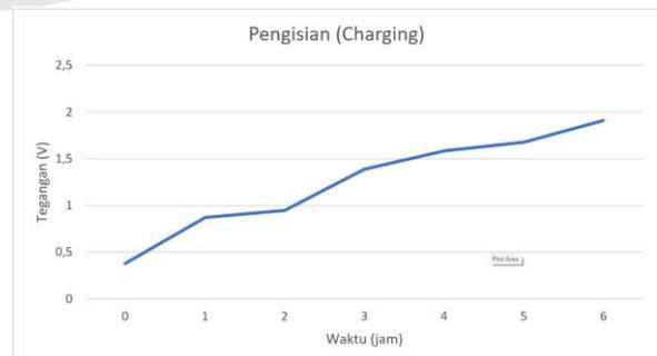
GAMBAR 17: GRAFIK HASIL PENGUJIAN PENGISIAN MODUL BATERAI ALUMINIUM
