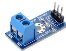
GAMBAR 2 Voltage sensor 0-25V
