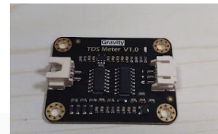
GAMBAR 2. DFRobot TDS Sensor
