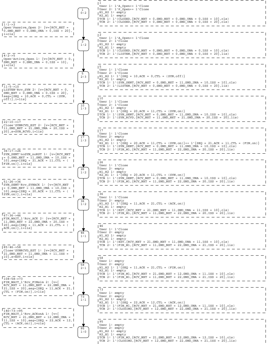
Fig. 5. A path in the occurrence graph for Configuration D (Model 1)
