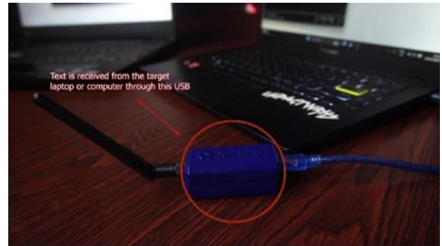
GAMBAR 4.6 Penerima USB keylogger
