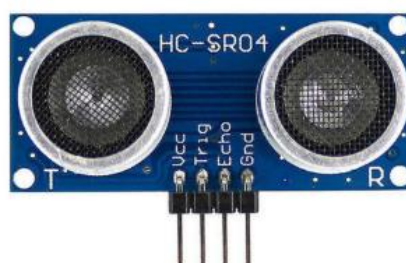
Gambar 2.1 Sensor Ultrasonik HC-SR04
