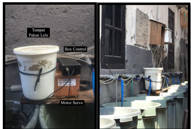
Figure 4 Automatic feed over 80 L bucket
