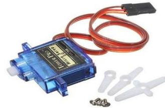
Gambar 2.2 Motor Servo Tipe Sg90
