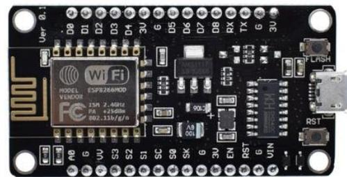
**Gambar 2.3** NodeMCU Esp8266 v3
