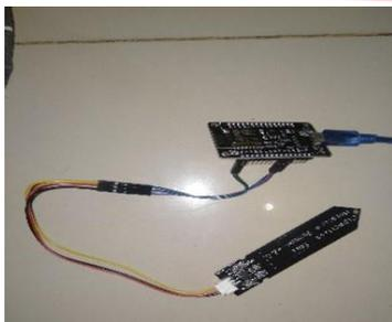
Gambar 4. 16. Pengujian capacitive soil moisture sensor
