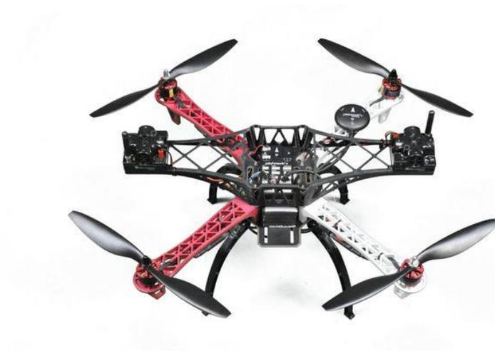
Gambar 2.1 Drone jenis Quadcopter [7]
