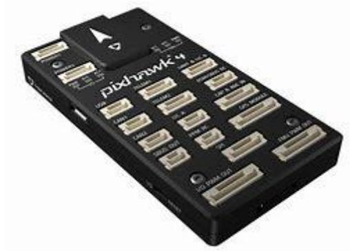
Gambar 2.5 *Flight Controller Pixhawk* [11]
