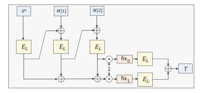
**Fig. 3.** The 1kf9 construction. It is built on top of a blockcipher  $E: \{0,1\}^k \times \{0,1\}^n \to \{0,1\}^n$  with a single key L.
