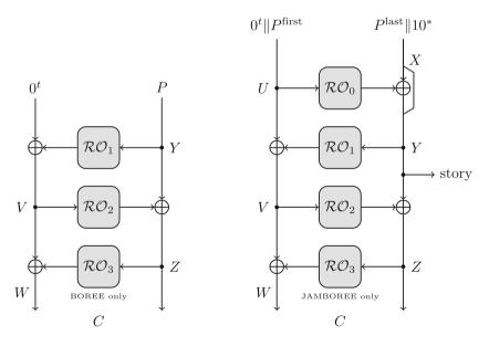
Fig. 1. Feistel network inside the different modes, Deck-BO(REE) on the left and Deck-JAMBO(REE) on the right.
