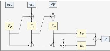
**Fig. 7. The n1kf9**[E] **construction.** It is built on top of a blockcipher  $E: \{0,1\}^k \times \{0,1\}^n \to \{0,1\}^n$  with a single key K.
