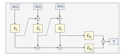
**Fig. 2.** The 3kf9 construction. It is built on top of a blockcipher  $E: \{0,1\}^k \times \{0,1\}^n \to \{0,1\}^n$  with three keys L,  $K_1$  and  $K_2$ .
