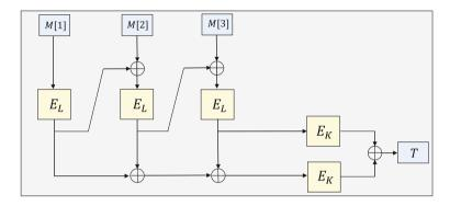
**Fig. 4.** The 2kf9 Construction. It is built on top of a blockcipher  $E: \{0,1\}^k \times \{0,1\}^n \to \{0,1\}^n$  with two keys L and K.
