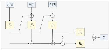
**Fig. 6. The n2kf9**[E] **construction.** It is built on top of a blockcipher  $E: \{0,1\}^k \times \{0,1\}^n \to \{0,1\}^n$  with two keys L and K.
