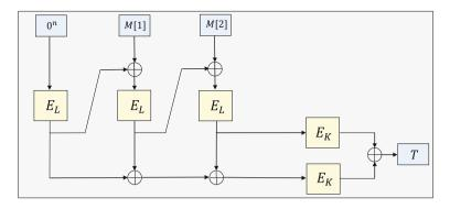
**Fig. 5.** A plausible construction. It is built on top of a blockcipher  $E: \{0,1\}^k \times \{0,1\}^n \to \{0,1\}^n$  with two keys L and K, and prepends an all-0 block at the beginning.
