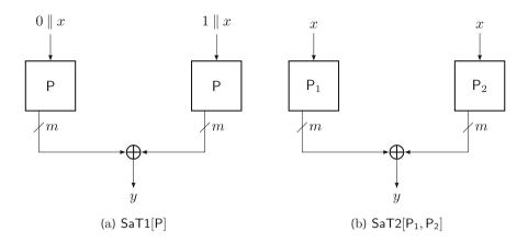
Fig. 1. SaT1 and SaT2 constructions
