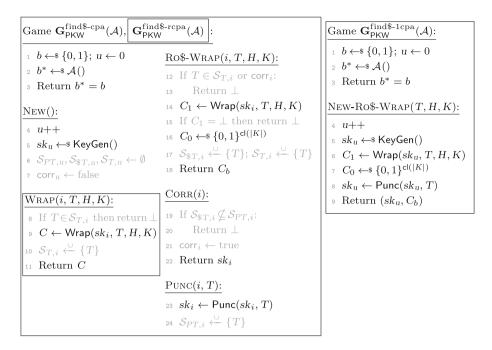
Fig. 3. Left and middle: Forward security and privacy find\$-cpa (without access to the boxed Wrap oracle)/find\$-rcpa (with access to Wrap) of a puncturable keywrapping scheme PKW. Right: One-time privacy and forward security find\$-1cpa security of a puncturable key-wrapping scheme PKW. Grey code prevents trivial attacks and ensures that unique tags are used for wrapping. (Color figure online)
