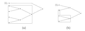
Fig. 3. The Counter-MGF construction instantiated via a tree hash function. The highlighted sub-trees are independent of the counter  $\langle i \rangle_l$ . We emphasize that the initial points represent the result of the compression between the initial value IV and the corresponding message block/ $\langle i \rangle$ .
