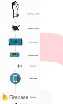
(Flowchart of How the Mobile Application and the Tool Work)
