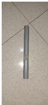
**Gambar 15** Pipa Kondisi Bocor Besar
