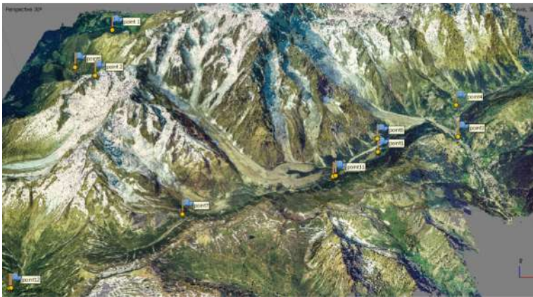
Fig. 3. An example of reconstructed 3D dense cloud from the 2001 dataset representing the position and distribution of GCPs.
