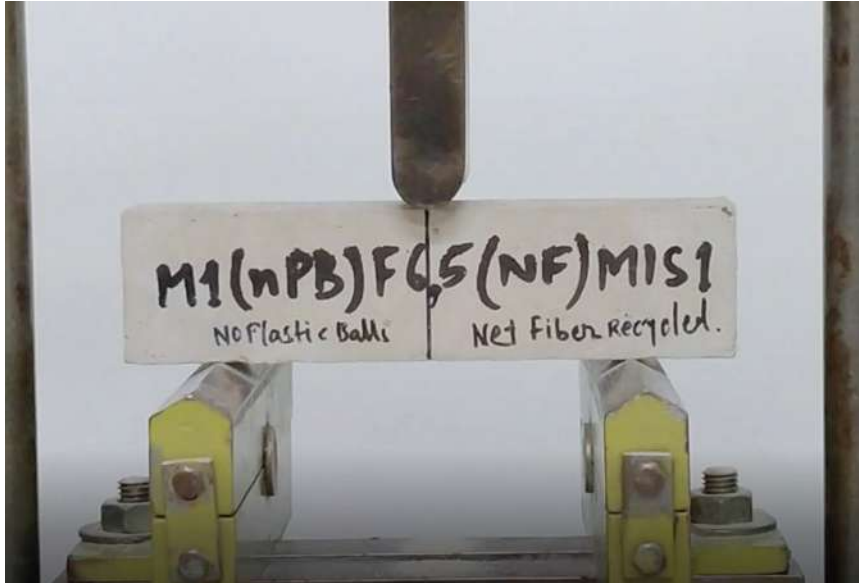
Fig. 5. Flexural strength test
