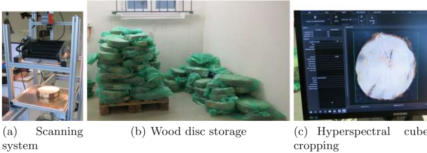
Fig. 1. The sensor system shows the line scanner which was mounted on a metal frame and the slice is moved perpendicular to the scanned line manually. The stored samples were closed airtight to avoid surface changes. Each hyperspectral cube was cropped to reduce the massive amount of data.
