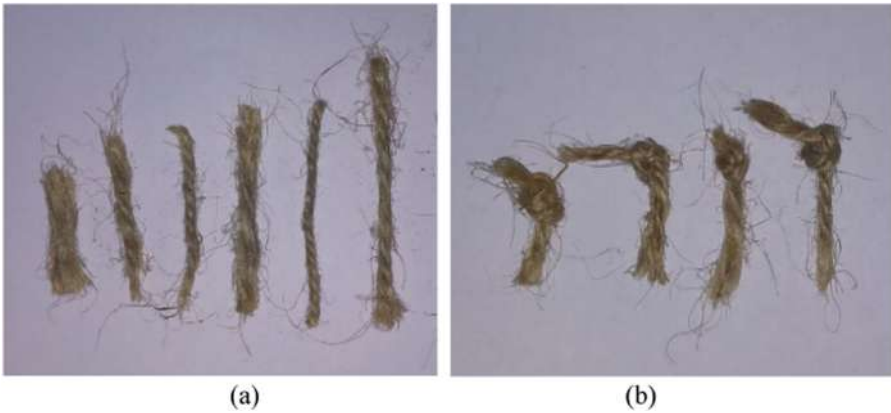
Fig. 3. (a) Thread fiber pieces of various sizes; (b) Presence of knots in some of the recycled jute net fibers
