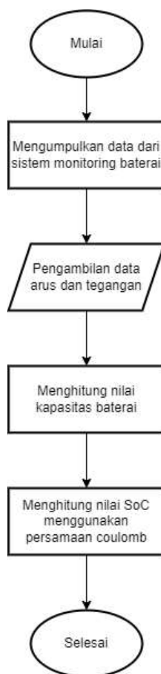
Gambar 1. 1 flowchart alur coulomb counting
