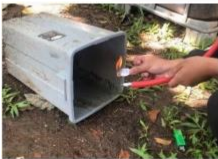
GAMBAR 3 Uji Bakar Gas Metana
