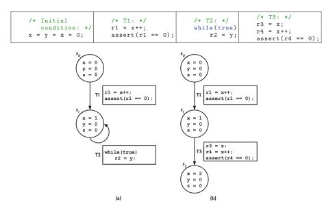
Fig. 1. Problem with existing stateful DPOR algorithms on a non-terminating multithreaded program. Execution (a) terminates at a state match without setting any backtracking points. Thus, stateful DPOR would miss exploring Execution (b) which has an assertion failure.
