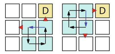
Fig. 2. Livelock patterns on a  $3 \times 3$  NoC.
