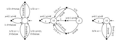
**Fig. 4.** Left: The coin game as a single-location PCFP  $\mathfrak{P}_{game}$ . Middle: The PCFP after unfolding variable  $\mathfrak{f}$ . Right: The PCFP after eliminating the location labeled  $\mathfrak{f}$ .
