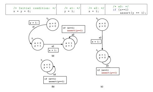
**Fig. 5.** Example of an event-driven program for which a naive application of the standard DPOR algorithm fails to construct the correct persistent set at state  $s_0$ . We assume that e1, e2, and e3 are all initially enabled.
