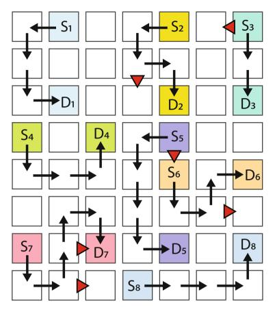
Fig. 1. Fault-tolerant routing examples. The black arrows show the path a packet will take; the red arrows point in the direction of a link fault. (Color figure online)
