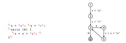
Fig. 3. Example of CFG generation.
