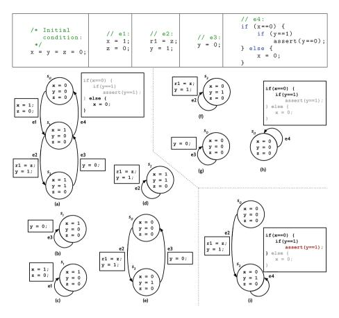
Fig. 3. Example of a event-driven program that misses an execution. We assume that e1, e2, e3, and e4 are all initially enabled.
