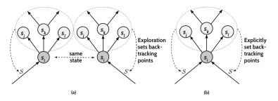
**Fig. 2.** (a) Stateless model checking explores  $s_i$ ,  $s_j$ ,  $s_k$ , and  $s_l$  twice and thus sets backtracking points for both S and S'. (b) Stateful model checking matches state  $s_i$  and skips the second exploration and thus we must explicitly set backtracking points.
