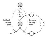
Fig. 4. Stateful model checking needs to handle loops caused by cyclic state spaces.
