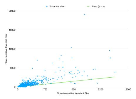
Fig. 5. Comparison of the number of variables introduced by the FIC transformation with the number of variables in a flow-insensitive analysis
