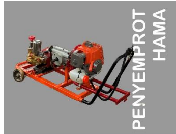
Gambar 3 Mesin Sprayer Implementasi Tractorpack
