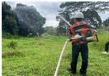
Gambar 4 Mesin Fire Pump Implementasi Tractorpack
