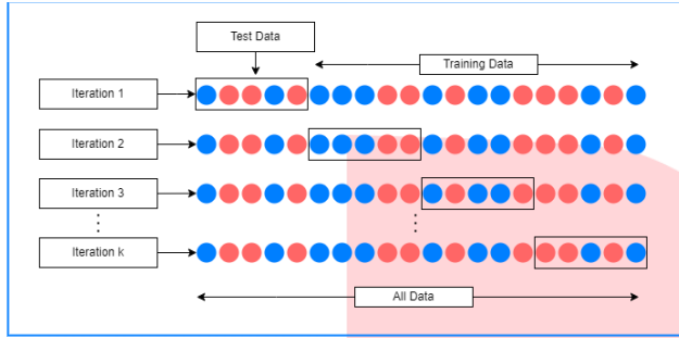
GAMBAR 2 Diagram K-Fold Cross Validation
