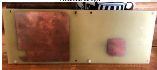
FIGURE 4 Front view fabricated antenna
