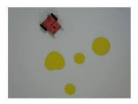
The destination point is symbolized by two small circles. More than one destination point is given to make it easier for the mobile robot to reach the final destination point.
