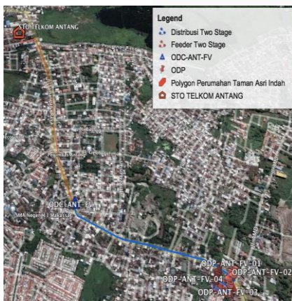
GAMBAR 5 Jalur Kabel Two Stage
