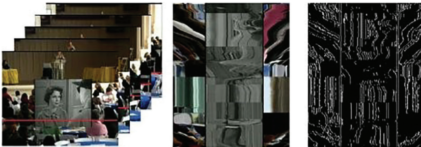
FIGURE 4.10 Synchronized feature vector based on video image detection. (a) A series of video frames. (b) Spatiotemporal slice. (c) Vertical edge image of (b).
