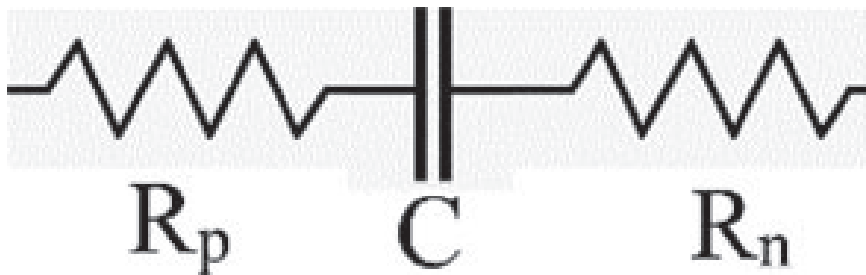
FIGURE 6.3 Simplified electrical circuit diagram for the proposed PIN phase shifter.
