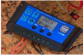
GAMBAR 2 (SOLAR CHARGER CONTROLLER)
