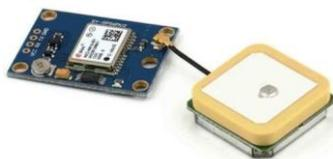
Gambar 3 Modul GPS Neo-8m
