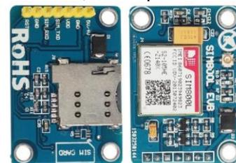
Gambar 2 Modul GSM SIM800L
