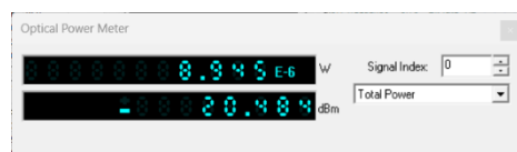
Gambar 4. 4 Hasil Power Received Terburuk Pada Link Akses Downstream
