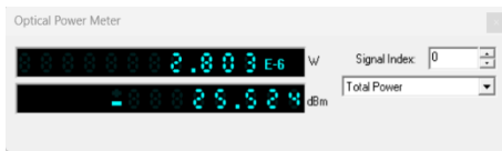
Gambar 4.2 Hasil Power Received Pada Link Backhaul
