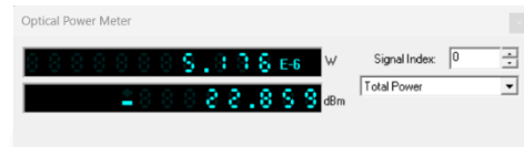
Gambar 4. 6 Hasil Power Received Terburuk Pada Link Akses Upstream
