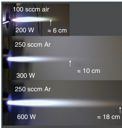
Figure 5.8 Comparison of lengths of the atmospheric plasma jets generated in air and in argon by the H-HEAD source without the contribution of the hollow cathode, see also Ref. [5.43].
