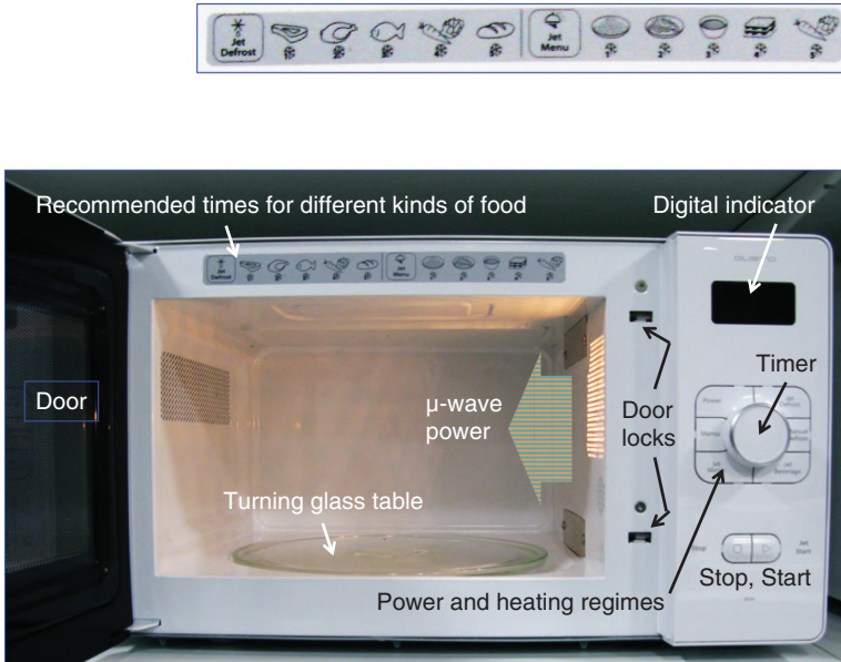
Figure 1.30 A view into a typical microwave oven with the power outlet arranged on the right side.
