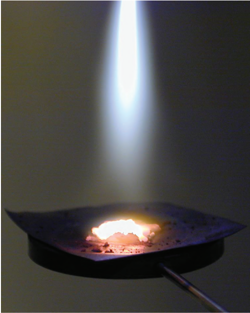
Figure 5.16 The H-HEAD plasma sintering of powders. Parameters on the photograph: 250 sccm Ar, 2.4 GHz, 400 W, hollow cathode pulsed DC 50 W, 0.5 \mu s, 250 kHz, 0.25 A. The substrate holder was 30 mm in diameter. The holder was fixed on 1.5 mm diameter stainless steel cartridge of the K-type thermocouple measuring the temperature of the substrate holder.
