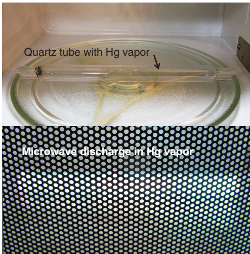
Figure 1.32 An illustration of the mercury (Hg) plasma generated by the microwave power inside the microwave oven. The discharge is shown behind the net-shielded door of the oven. The intensity of the discharge is not uniform and it depends on the position of the table.
