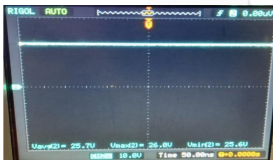
Gambar 12 Grafik osiloskop dioda bridge 3A
