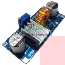
GAMBAR III. 2 Modul Buck Converter Step Down
