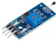
GAMBAR II.4 Modul NTC Thermistor
