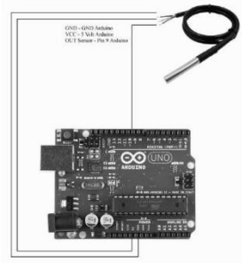
GND Sensor Suhu GND Arduino VCC 5Volt Arduino OUT Sensor Pin 9 Arduino
