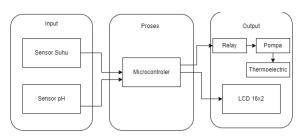
Figure 2. 2 Block diagram of Automatic Water Temperature and Water Stability Control System
